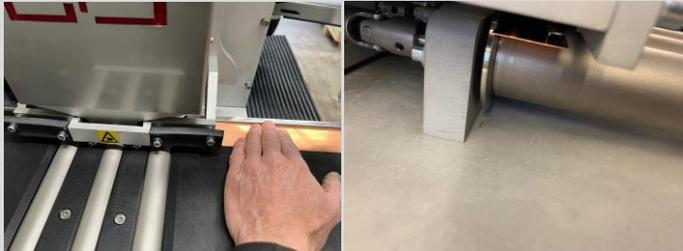
Remove the hands from sample and press the right foot pedal to transport the strip sample underneath the measuring head. When measuring wider strip samples there might be need to assist the strip feeding slightly by pushing the sample, by holding the opposite edge to what is currently being measured.
